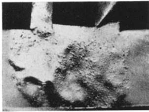
Appearance of vapour blanket at end of heating pulse
