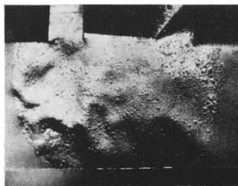
FIG. 12. Event sequence in which target reaches 500°C at 80°C subcooling.
